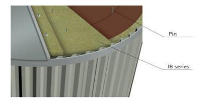
To avoid thermal bridge, the two layers of RK series products should be secured tightly at all lateral and longitudinal joints of each layer, and the joints of two layers should be staggered at about 150 mm;
