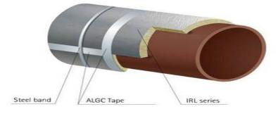
The blankets are secured with two steel banding at about 100 mm from the lateral joints and should be covered with profiled aluminum sheet to protect them from mechanical or weather damage.
